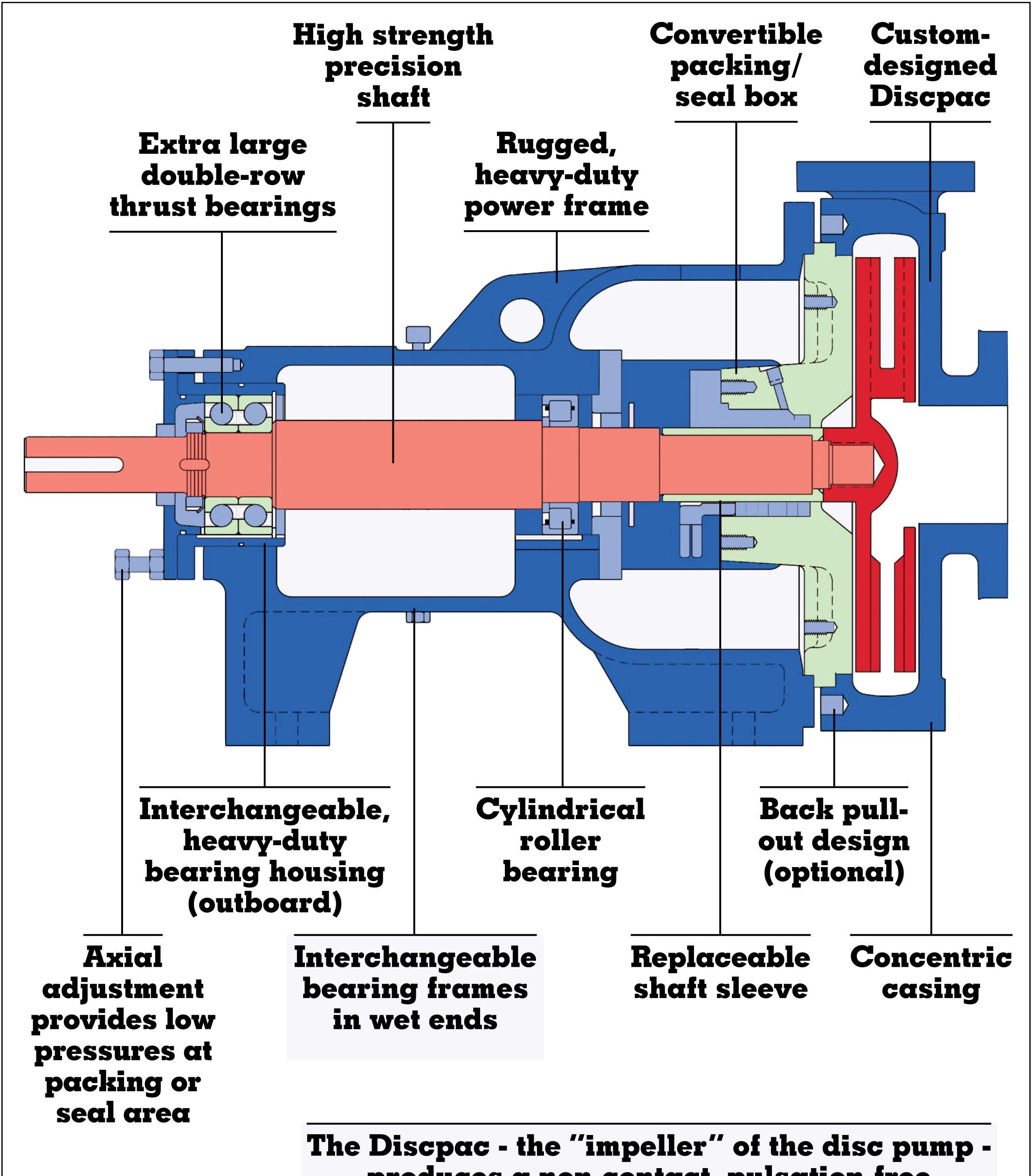
The Discpac - the "impeller" of the disc pump produces a non-contact, pulsation-free pumping action, making the pump ideal for hard-to-pump applications.
