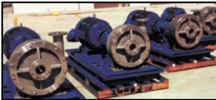
Titanium pumps used for handling hazardous chemicals are on their way to a manufacturing plant in South Carolina.
